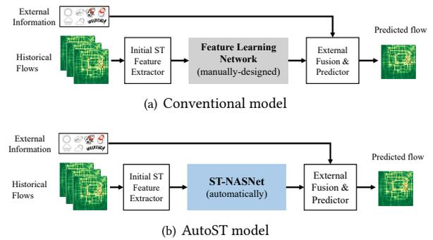
**Figure 2: Conventional model vs. our AutoST model**
